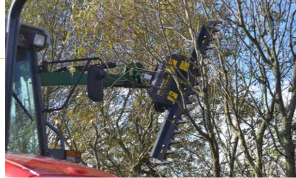
▲ Branch cutting with the SP23 cutterbar
